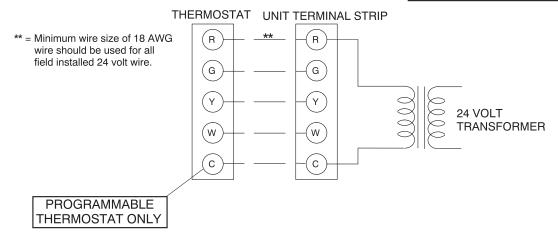
FIGURE 3 - TYPICAL FIELD CONTROL WIRING DIAGRAM
